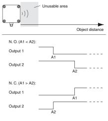
A1  $\rightarrow \infty$ , A2  $\rightarrow \infty$ : Object presence detection Both outputs are active if Object within detection range.
